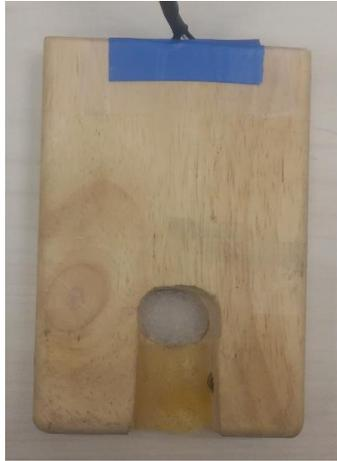
The Optic TapPad enables fine fast and quiet tapping with one finger (as opposed to the keyboard or the response box). It operates with a LED light on one side and a photo-diode on the other, and each time the participant “taps” the light-beam is broken and the photo-diode does not sense the light.
